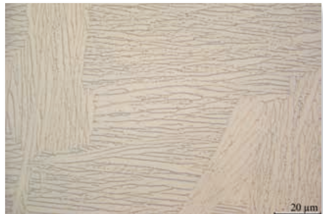
Fig. 6 Magnified view of the lamellar structure of Tilastan® TiAl6V4 immediately after casting.
