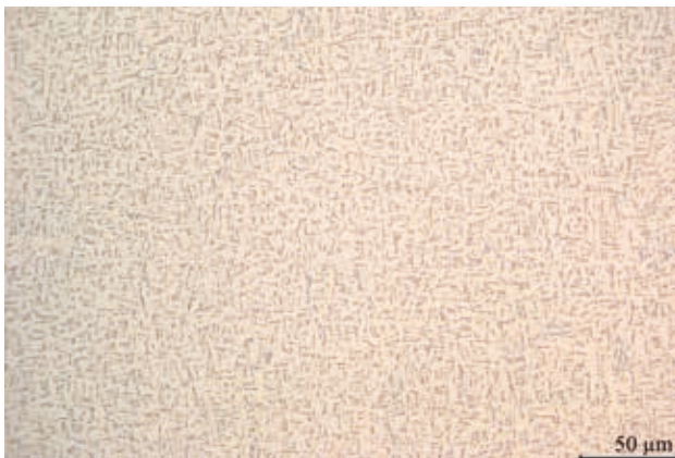
Fig. 16 After refinement by means of HIP and thermochemical heat treatment, the VACUCAST® titanium components have a very fine lamellar microstructure.
