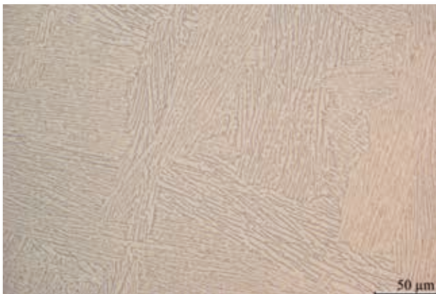
Fig. 11 Following HIP treatment, the structure of both the cobalt-chrome (9, 10) and titanium components (11, 12) is pore-free. Initial homogenization of the structural components has already occurred under the influence of the heat, this is evident by the broken lamellar structure.
