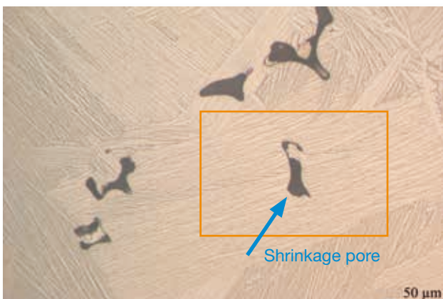
Fig. 7 The structure of TiAl6V4 is characterized by its lamellar nature comprising a \alpha matrix and \beta phases. Possible casting pores are markedly different from the microstructure.
