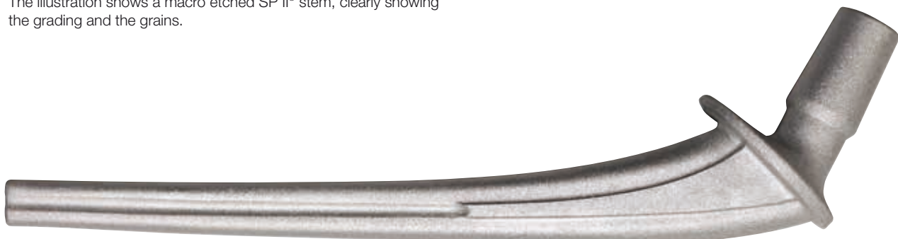
Fig. 21 The above macro etched SP II® stem shows the ideal fine-grained Biodur® structure.
