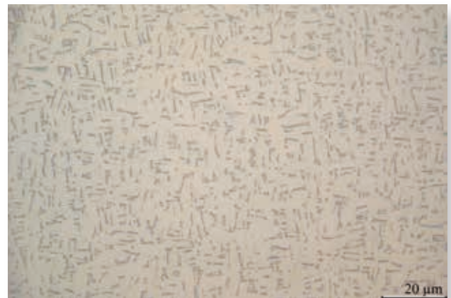
Fig. 17 Enlarged view of Fig.16 The \alpha + \beta alloy has a basketweave structure here.
