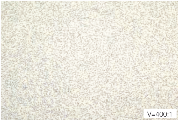
Fig. 18 Compared to a globular (Fig.18) or bimodal forging structure (Fig. 19), the VACUCAST® cast structure (Figs. 16 and 17) has a minimal tendency for crack propagation due to its very fine basketwork lamellar structure.
