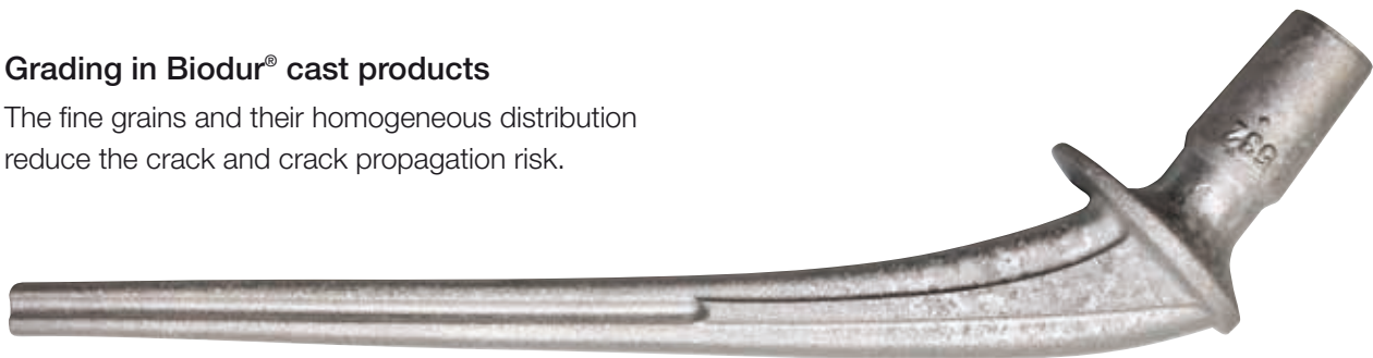
Fig. 20 The illustration shows a macro etched SP II® stem, clearly showing the grading and the grains.
